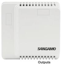
**General Information** Dimensions (mm) 78 x 78 x 36 Finish White Sensor Type Bi-Metallic Sensing Element Materials ABS Weight (Kg) 0.16 Warranty (Years) 3 **Programming** Set Temperature Range (°C) -5 to 30 **Supply & Power** Supply Voltage (V AC) 230 IEC Protection Class II **Environment**
