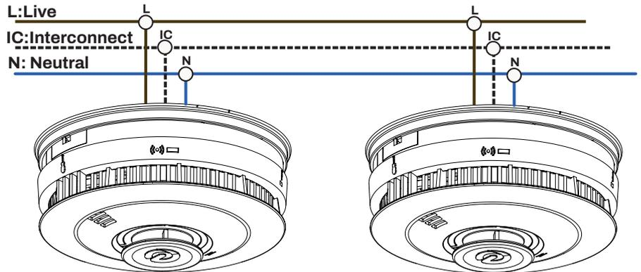
Heat Alarms must always be interconnected to a smoke or multi-sensor Alarm to ensure early warning.
