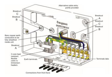
The Powersaver Dual Flexi should be removed from the mounting box by unscrewing the 2 captive pattress screws.
