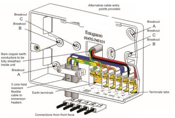
The Powersaver Dual Flexi should be removed from the mounting box by unscrewing the 2 captive pattress screws.
