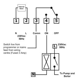
Choice Rstat3-RF receiver used in a conventional fully pumped system using a 2 port spring return valve with auxiliary switch to control the pump and boiler. Note: Hot water will need to be controlled by the use of a programmer or timeswitch.
