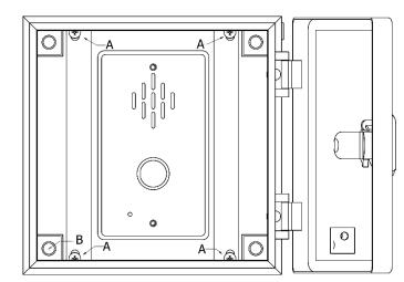
The enclosure can now be prepared for the cable from the EVC System, this is a 2 core 1.5mm CSA fire rated cable\*.
