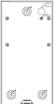
The Back box can now be mounted by using the holes marked B, the height of
