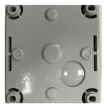
There are 8 screw mounting positions which are shown in the photo on the left. It should be noted that the IP rating will be affected if the internal fixing point are used. To keep the IP-56 rating the four external fixing points located in the corners should be utilised.
