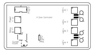
The terminals on the BA4ZMPS are marked "12V out" 0 & +V, which should be connected to the terminals marked power 0 & + on the BA4ZM
