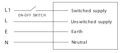
L1 is the transition switch for maintained mode if required.
