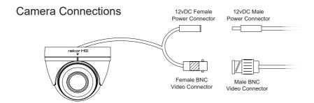
Please Note: The camera housing is suitable for outdoor use (Ingress Protection: IP66). The Power & Video connections are required to be made internally or in a suitable ingress protected box.
