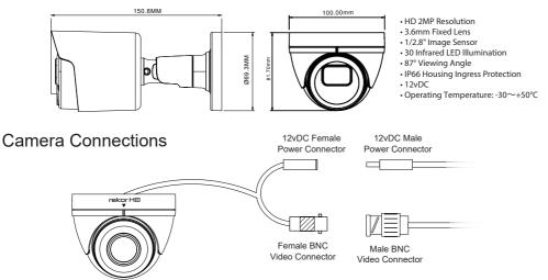
Please Note: The camera housing is suitable for outdoor use (Ingress Protection: IP66). The Power & Video connections are required to be made internally or in a suitable ingress protected box.
