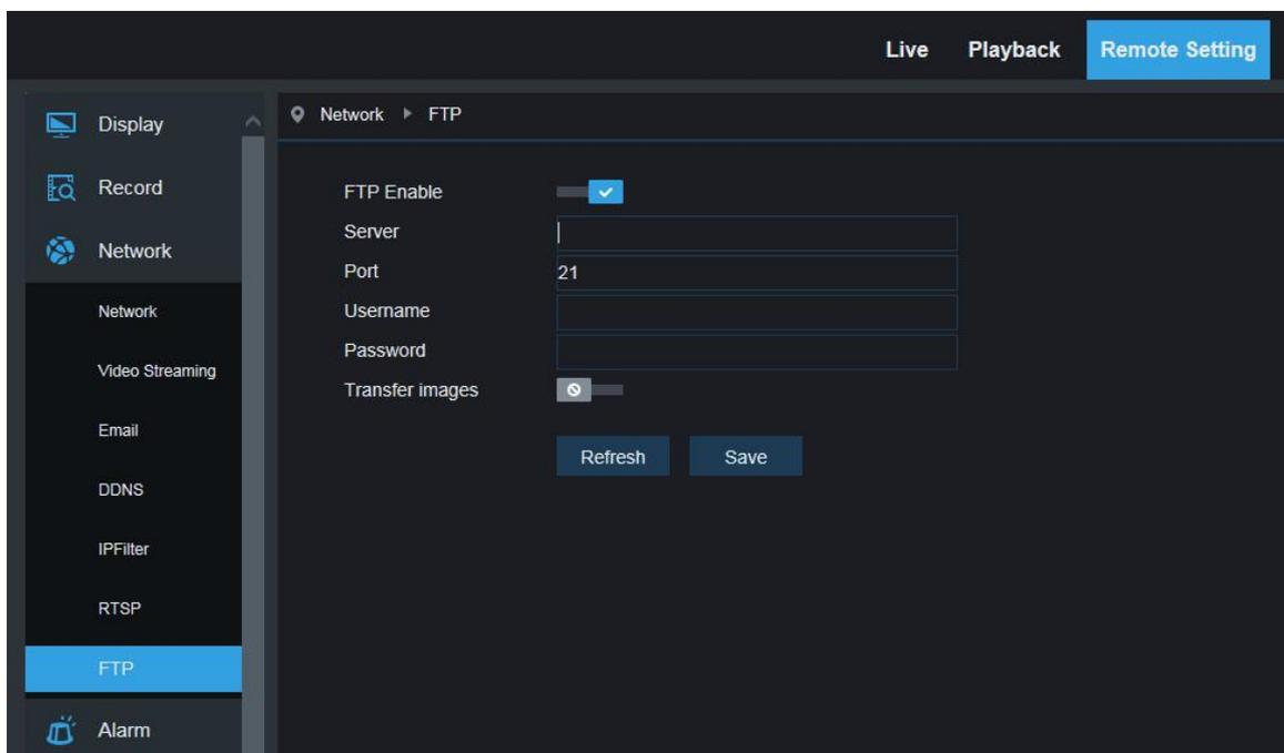
**FTP:** FTP service setting - used with alarm function to upload images or videos snapped to the FTP server.
