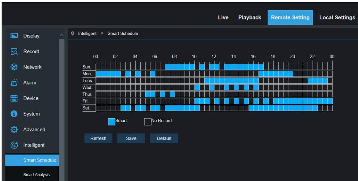
one grid in the table is 30 minute, User can setup according to private requirement to choose different record type and time.
