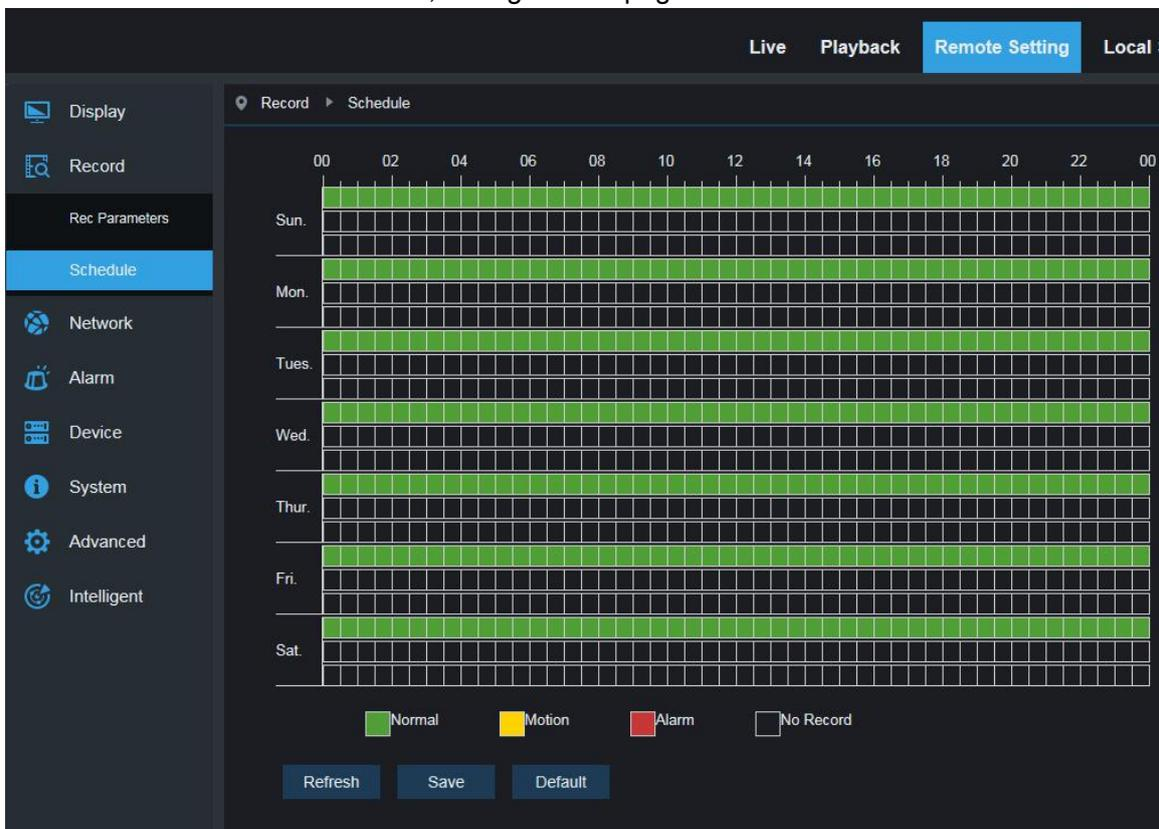
As image: one grid in the table is 30 minutes, green is normal record, yellow is motion detection alarm, red is I/O. User can setup according to private requirement to choose different record type and time.
