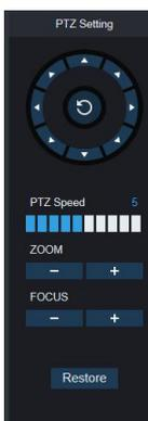
: It has eight difference angle to control in the circle button , 0-10,it means difference PTZ speed, ZOOM:adjust lens FOCUS: fix lens.Restore: restore factory setting .
