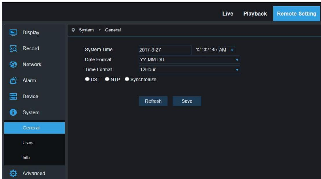
The device time, system time, date format and time format contained in the basic information can be manually set and saved.
