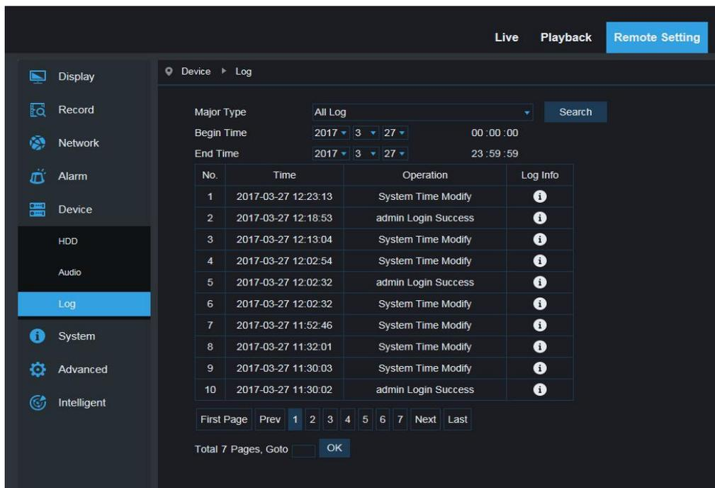
**Log Type:** Eight types of logs are available - system logs, network logs, parameter logs, alarm logs, user logs, recording logs, storage logs and all logs). Choose the starting and ending date/time for retrieval.
