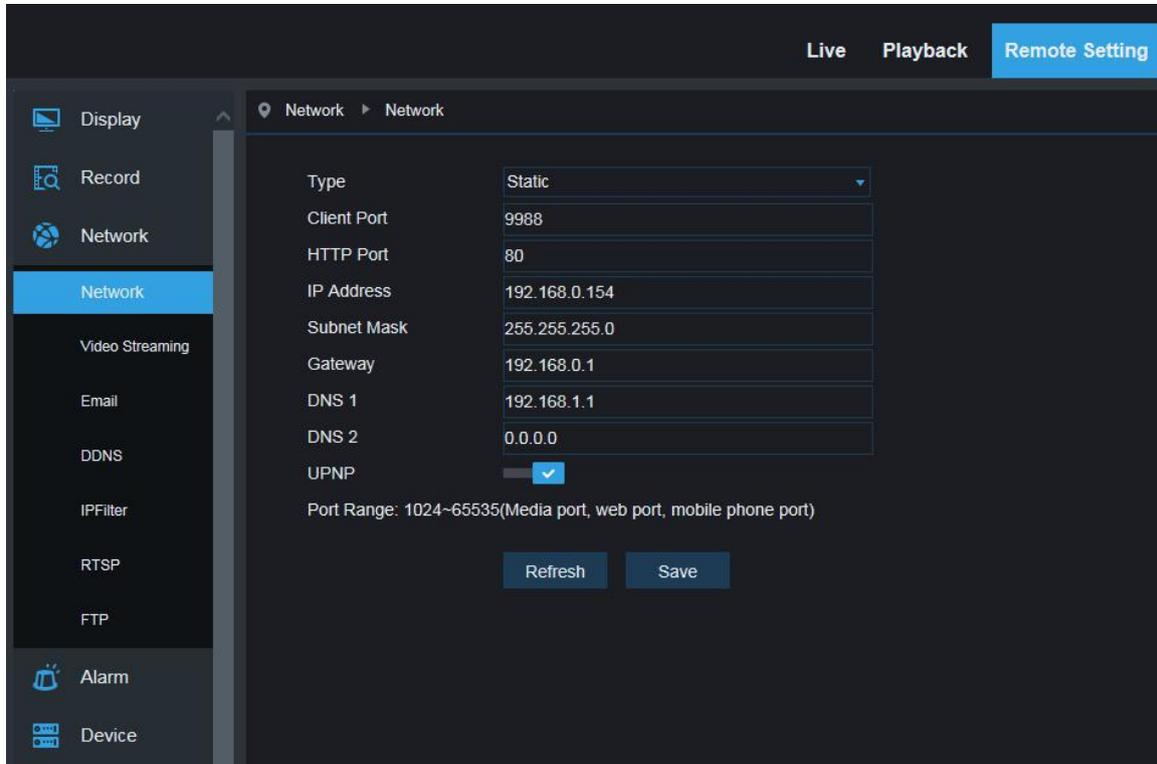
**Networking mode:** DHCP (Automatically Acquired), Manually Configured and PPPOE; the default is Manually Configured
