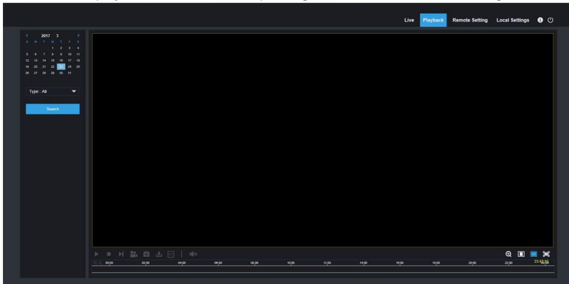
User can search video by file type as needed, and operate the video through the simple tool on the toolbar, e.g. open/stop video , bit stream video, recording, snapshot, download recording , quick motion video playback, Sound On/Off.
