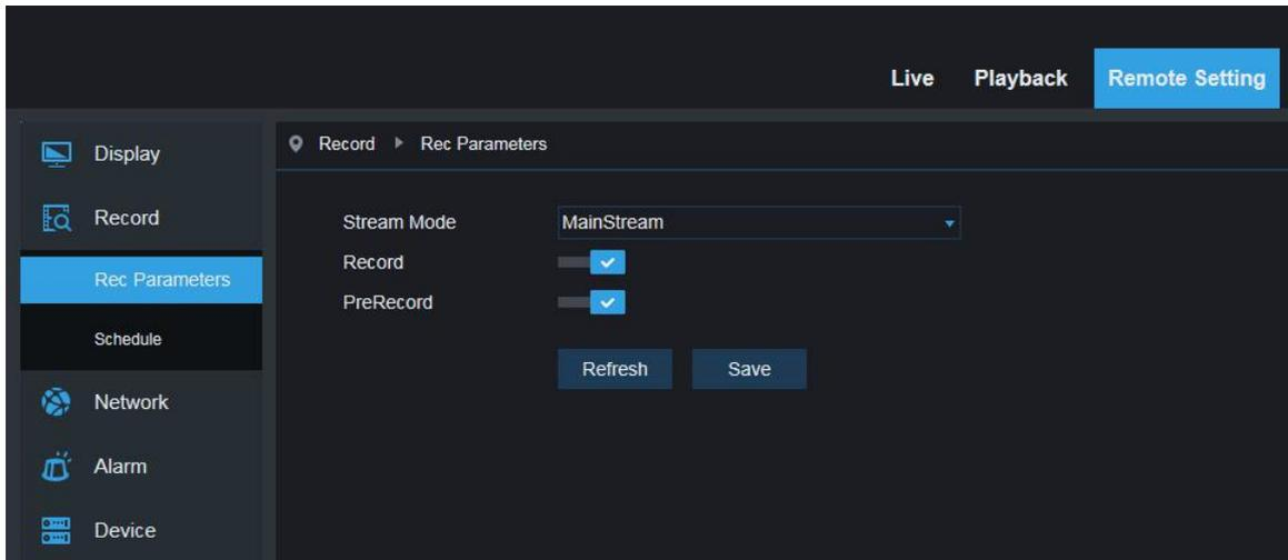
This function is to control the record, pre record and record type (main stream and substream)
