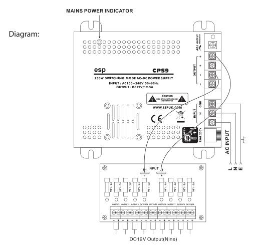
Note : Total maximum power loading not over 12.5Amp at 12VDC
