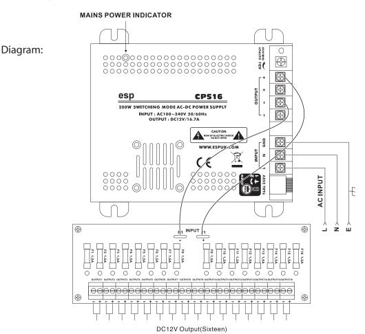
Note: Total maximum power loading not over 16.7Amp at 12VDC
