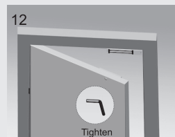
12 Tighten the tamper screw after making sure all installation steps are correct and work well.
